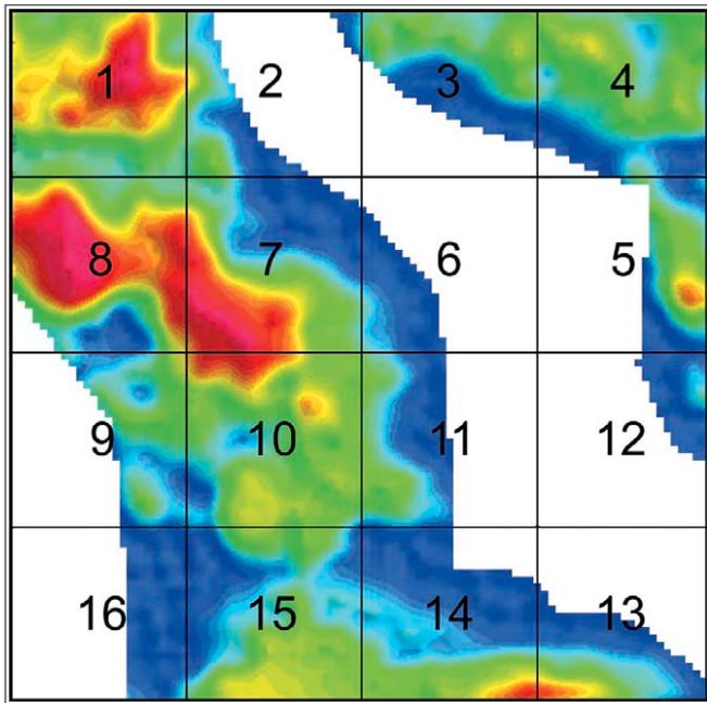
**Figure 7.** Shallow salt isopach—a salt thickness map based on the seismically interpreted top of salt horizon and the 3D earth model interpretation for the base of the shallow allochthonous salt. The results met premodel expectations, showing a salt body varying in thickness from 1500 to 5000 m. Two surprises were found: a deep salt root north and west of the prospect proper, and the rugosity of the salt base.
