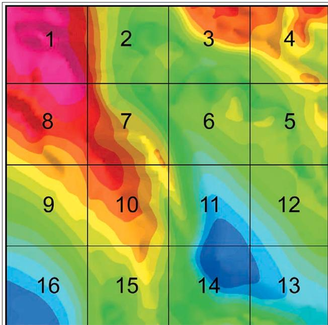
Figure 3. Bathymetry was supplied by Kerr-McGee as a water bottom depth file in digital form. The depth has been referenced to sea level. The seafloor topographic relief varies across the area between 1040-1640 m.
