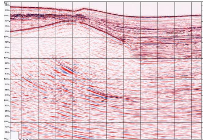
Figure 1. Seismic section illustrates the problem of determining the base of an allochthonous salt mass. The deeper reflectors show the possibility of the sedimentary section under the salt, but how far laterally and at what depth does it truncate against the salt are questionable (Seismic section courtesy of Veritas).
