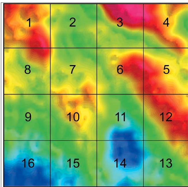
Figure 4. The Bell tensor gradient field  $T_{zz}$  is shown above. It is one of six tensor gradients ( $T_{xx}$ ,  $T_{yy}$ ,  $T_{zz}$ ,  $T_{xy}$ ,  $T_{xz}$ , and  $T_{yz}$ ), which covered a  $4 \times 4$  OCS block area surrounding the prospect. It is considered as one of the key tensors used in this interpretation.
