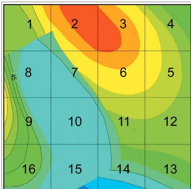
**Figure 6.** IGC basement surface interpreted from FAS aeromagnetic data as the depth to the top of crystalline or igneous crust. From a regional perspective, the 16 block area of interest lies on the north half of a broad, subcircular basement platform. Subsea depth ranges from 40 000 (red) to 46 000 (light blue) feet.
