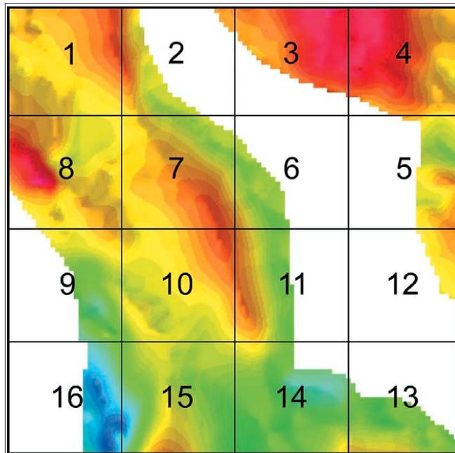
Figure 5. Kerr-McGee top of salt horizon interpretation was seismically derived. The surface covered the 16 blocks of interest with considerable overlap blocks to avoid limiting the areal extent of the 3D earth model. Null zones indicated were interpreted as areas deprived of the shallow allochthonous salt.
