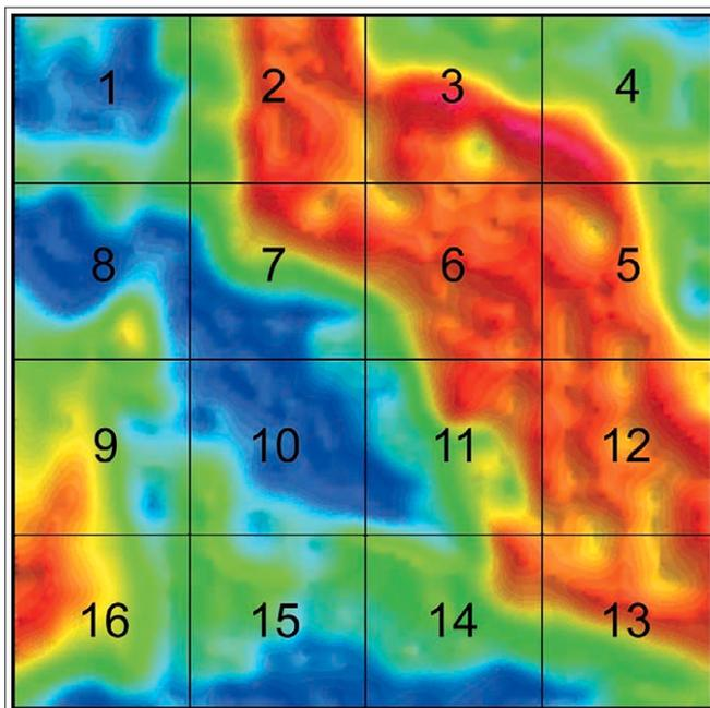
**Figure 8.** Sediment isopach—an interpretation map from the 3D earth model results delineates the varying thickness of sediment section existing between the allochthonous and autochthonous salt bodies.
